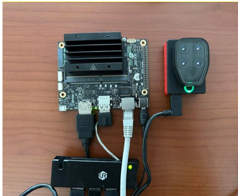
Figure 26: Connection of Sequoia with Jetson-Nano.
