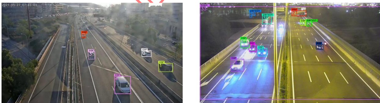
Figure 3: Work: Detection and tracking using siamot for detecting vehicles in a highway at daytime with backlight (left) and at night time (right), small objects are not detected and the approach is not correctly working with poor light conditions.
