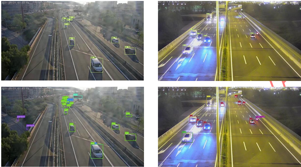
Figure 4: Figure cmp_yolo_efficientDet: Results comparison between EfficientDet (top) and Scaled-YOLO_v4 (bottom) approaches at daytime with backlight (left), and at night time (right). Better results are achieved using scaled-yolo_v4 in general.
