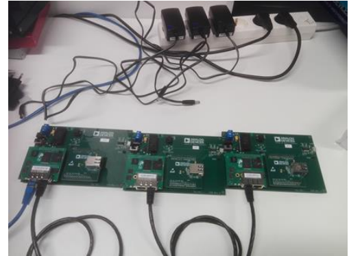
Figure 4-4 Lab measurements TSN synchronization
