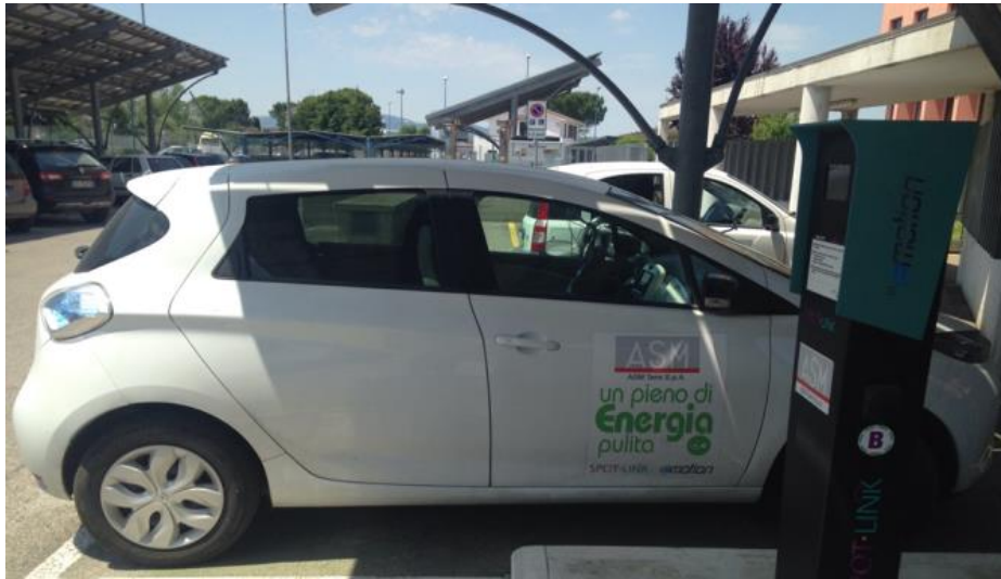
Figure 12: EVSE (Electric Vehicle Supply Equipment).
